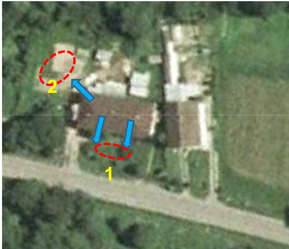
Rainwater garden 2: dimensions - 10 x 5 m area - 40 m 2 location on plot number 24/2
